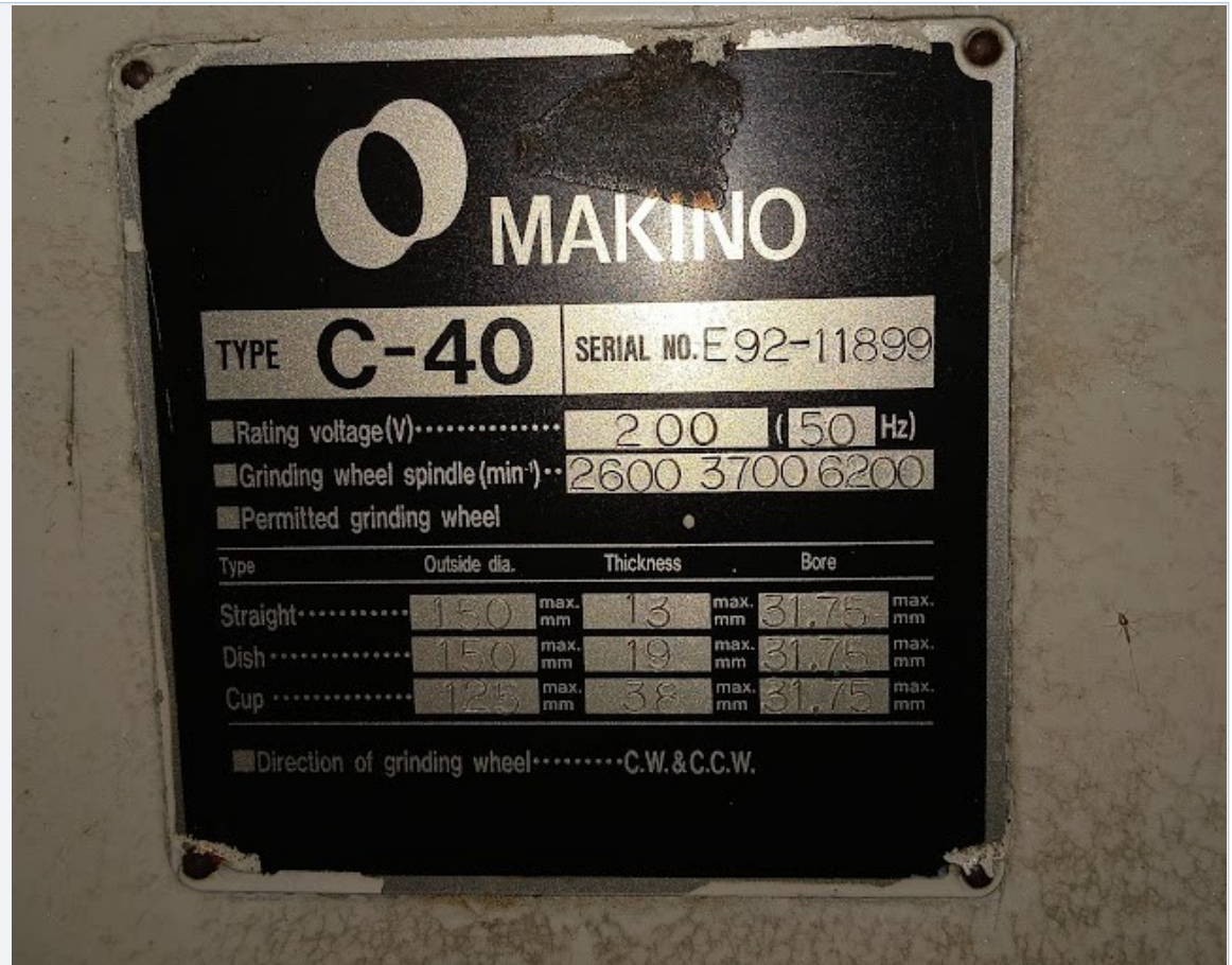
Nameplate: power and wheel specifications
