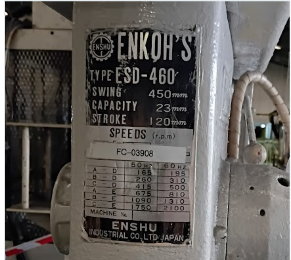
Nameplate: capacity and speeds
